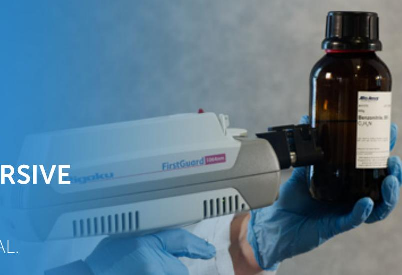
Increased capability for identifying genuine versus counterfeit materials is achieved by using dispersive 1064nm Raman analyzers.
