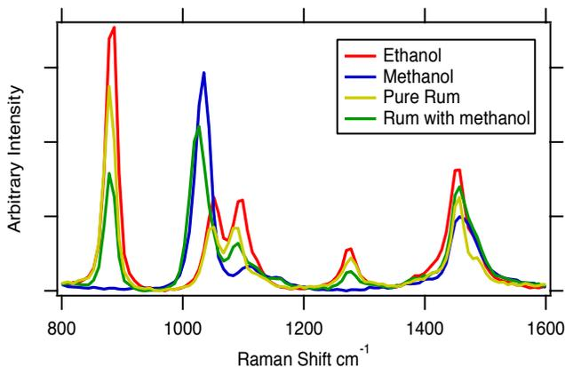
Figure 1: 1064 nm Raman spectra showing the difference between Rum with and without methanol.
