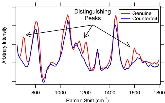
Figure 2: Raman spectra of genuine and counterfeit shampoos measured with 1064nm excitation.
